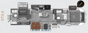
**LENGTH** 39'9-1/2" | **HEIGHT** 13'6" | **SLEEP CAPACITY** 5-6 **HITCH** 3,136 LBS | **DRY WEIGHT** 13,194 LBS | **GVWR** 15,000 LBS
