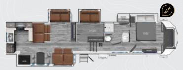
**LENGTH** 41'9" | **HEIGHT** 13'6" | **SLEEP CAPACITY** 7-8 **HITCH** 2,623 LBS | **DRY WEIGHT** 12,823 LBS | **GVWR** 15,000 LBS
